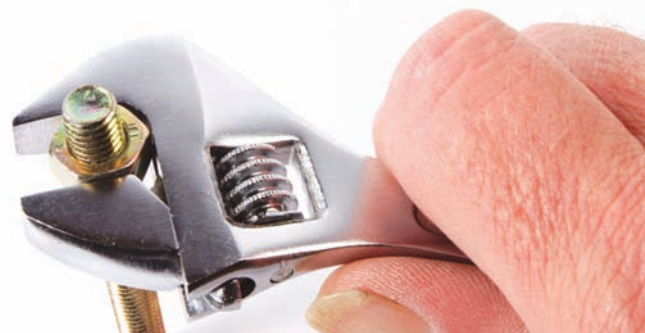
Figure 4.19 A wrench makes it easier to remove a nut from a bolt.
