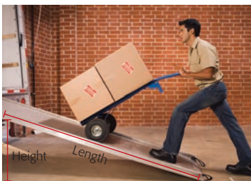
Figure 4.22 The length of the ramp is greater than the height of the truck. By using a ramp to do the work over a longer distance, the person uses less force.
