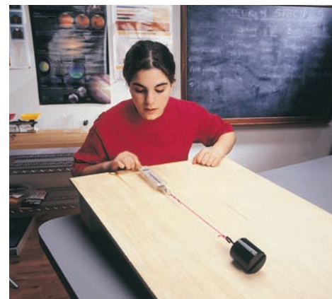
Figure 4.11 Spring scales can be used to determine the force required to move an object.
