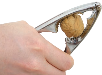
Figure 4.21 The force that the jaws apply to the nut is greater than the force that the person applies to the handles.
