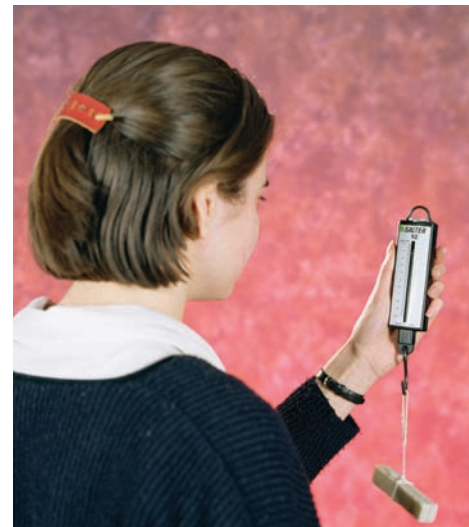
Figure 4.10 The spring scale shows the weight of an object in newtons.
