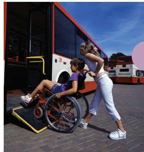
Figure 4.25 The ramp has a mechanical advantage greater than 1 since the force needed to push the wheelchair up the ramp is less than the force needed to lift the wheelchair straight up.
