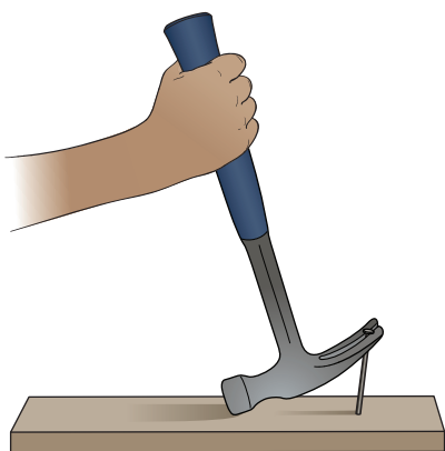
Figure 4.27 The ideal mechanical advantage of the hammer can be determined by comparing the distance the handle moves to the distance the nail moves.
