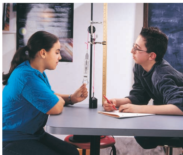
Figure 4.26 Machines that have a mechanical advantage of 1 only change the direction between the input and the output forces.
