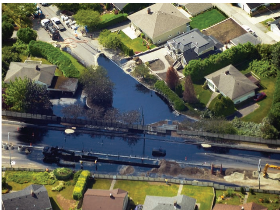
Figure 9.26 A major spill of crude oil occurred in Burnaby, British Columbia, on July 24, 2007. An excavator accidentally broke a crude oil pipeline, causing 240 000 L of oil to be released. The spilled oil coated the ground, vehicles, and homes.
